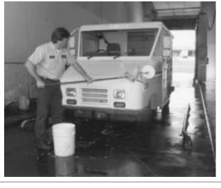
removed, these systems use any combination of cold water, hot water, or steam, with no detergent, heavy duty detergent, or acid-detergent washes. When necessary, vehicles are brushed to remove mud and dirt before the high-pressure water system is utilized. Washing times vary depending on the equipment used, how dirty the vehicle is, and how clean the vehicle needs to be. Typical washing times are approximately 10 minutes to wash an LLV and up to 30 minutes to wash a tractor-trailer.
